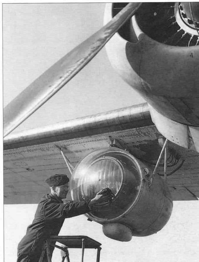
Right: A Leigh Light installation on a Vickers Wellington bomber of Coastal Command. These powerful searchlights were used to illuminate U-boats attempting to cross the Bay of Biscay under cover of darkness. Even surfaced U-boats could be very difficult to spot.
