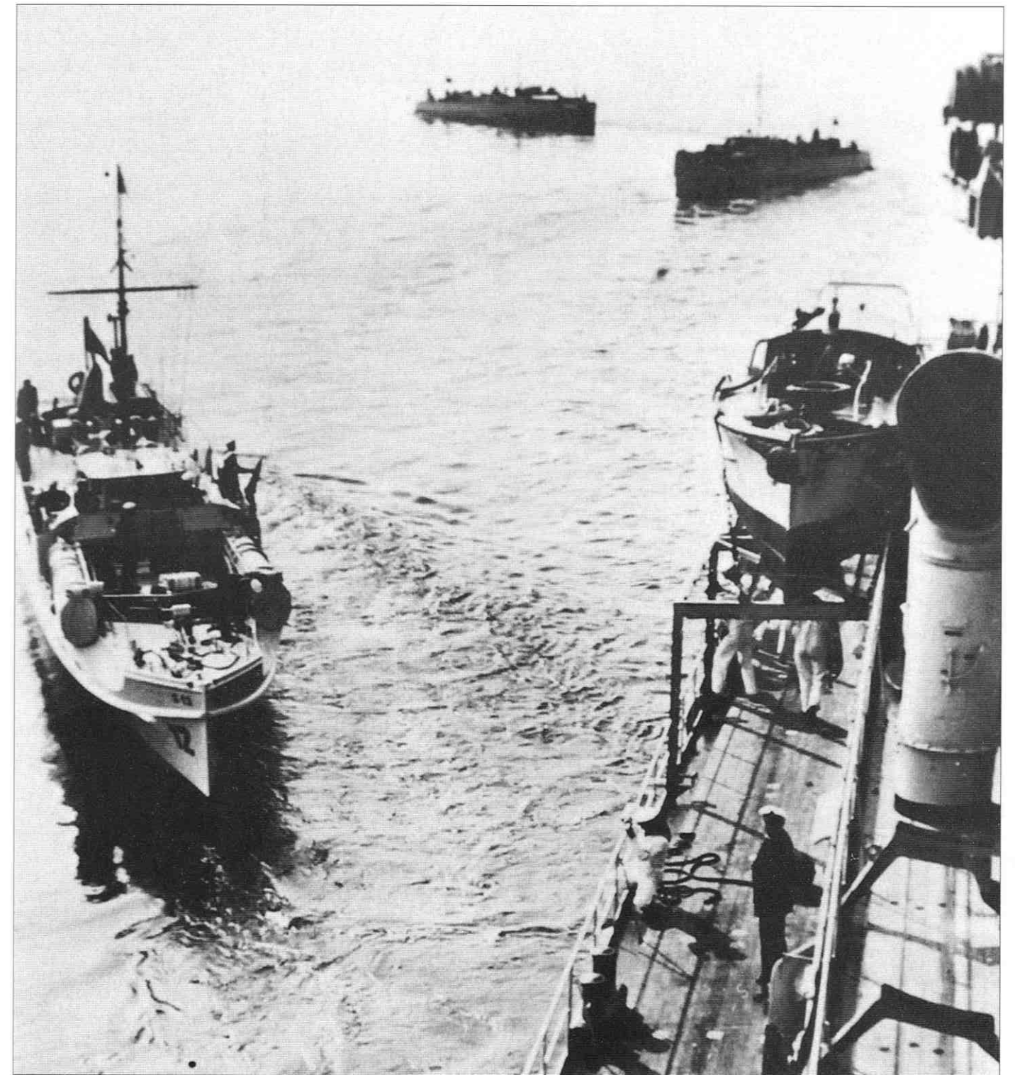
Above: S12 approaching its depot ship. This S-boat was one of a batch of four built in 1934 at the Lürssen shipyard, Vegesack. They displaced 78 tons and had a 21-man crew. Original armament was a single 20mm AA gun and two torpedo tubes.
