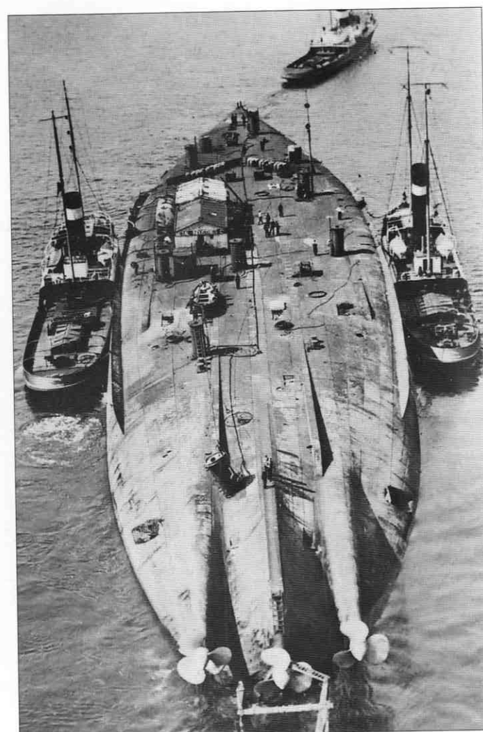
Above: The Kaiser-class dreadnought Kaiserin being broken up at Rosyth in 1936 after salvage. The vessel is still inverted. Note the massive turret for her twin 30.5cm (12in) guns. Kaiserin was one of the first German battleships to be fitted with turbines.
