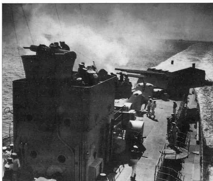
Below: The Königsberg in action. Light cruisers of this class carried a main armament of eight 5.9in (150mm) guns and a secondary anti-aircraft armament. They had a combat radius of 5300 miles (8527km) at 18 knots.
