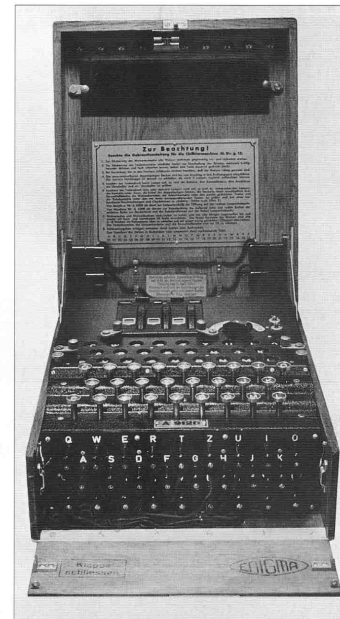
Above: The prototype Enigma code-machine, first developed by Dr Arthur Scherbius in 1923. The possession by British intelligence of the Enigma naval code played a significant, if not decisive, part in winning the Battle of the Atlantic, and also in the defeat of the Italian Navy in the Mediterranean.
