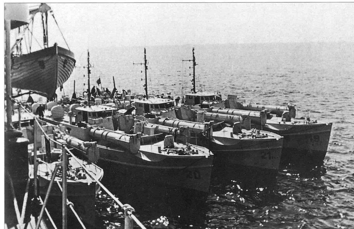
Above: S-boats moored alongside a depot ship. The German MTBs were between 80 and 100 tons in displacement, had crews of up to 25 men and, with their three diesel engines, could reach speeds of between 36 and 40 knots.
