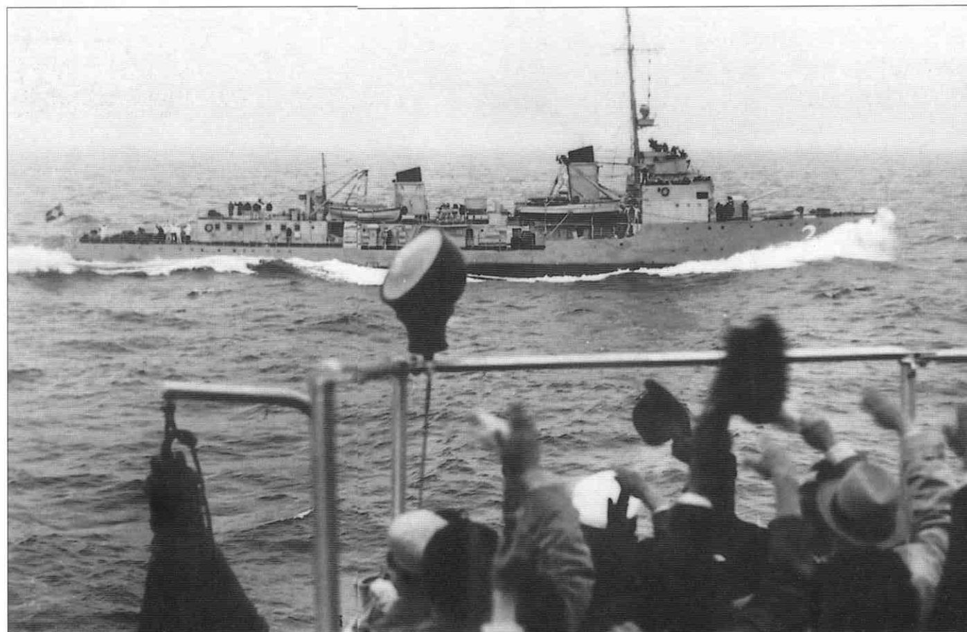
Above: Atlantic waves crash over the bow of an F-class escort vessel. There were 10 ships in this class, launched in 1945, but their complicated machinery gave so much trouble that they were never used in their intended role.
